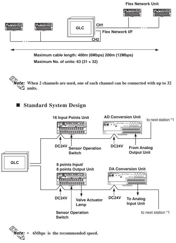
\*1 Be sure the Terminal Switch (TERM) of the network's last unit (at each end) is turned ON.
