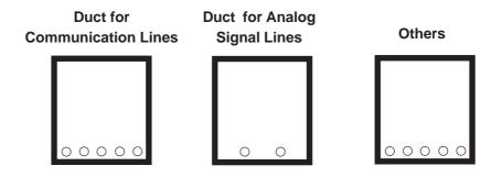
If the wires must be placed in the same duct, separate them via an earthed/ grounded divider.
